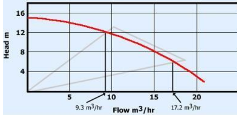
Example Pump Performance Curve
